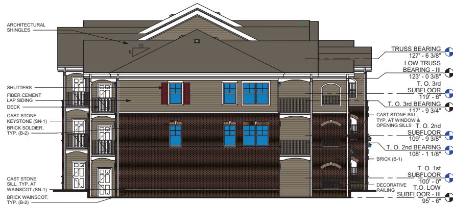
4 BLDG 11 - TYPE III - SIDE ELEVATION 1 1/8" = 1'-0"
