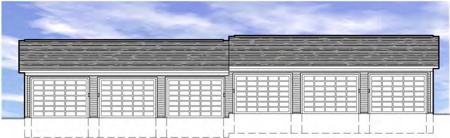
6-Stall Front Elevation w/ 2 Finish Floor Elevations
