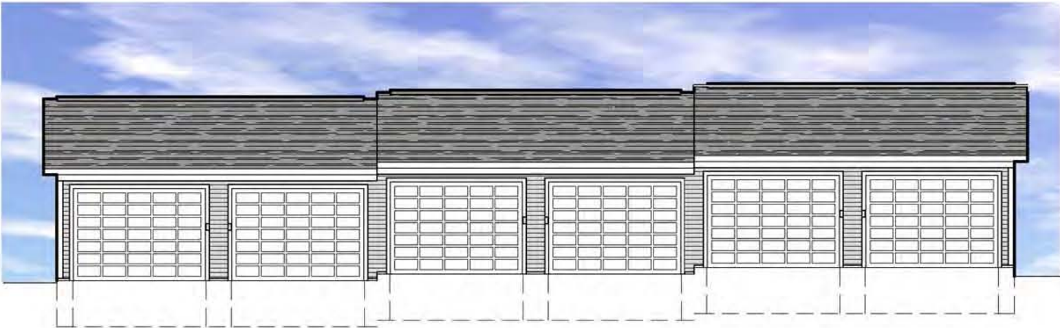
6-Stall Front Elevation w/ 3 Finish Floor Elevations
