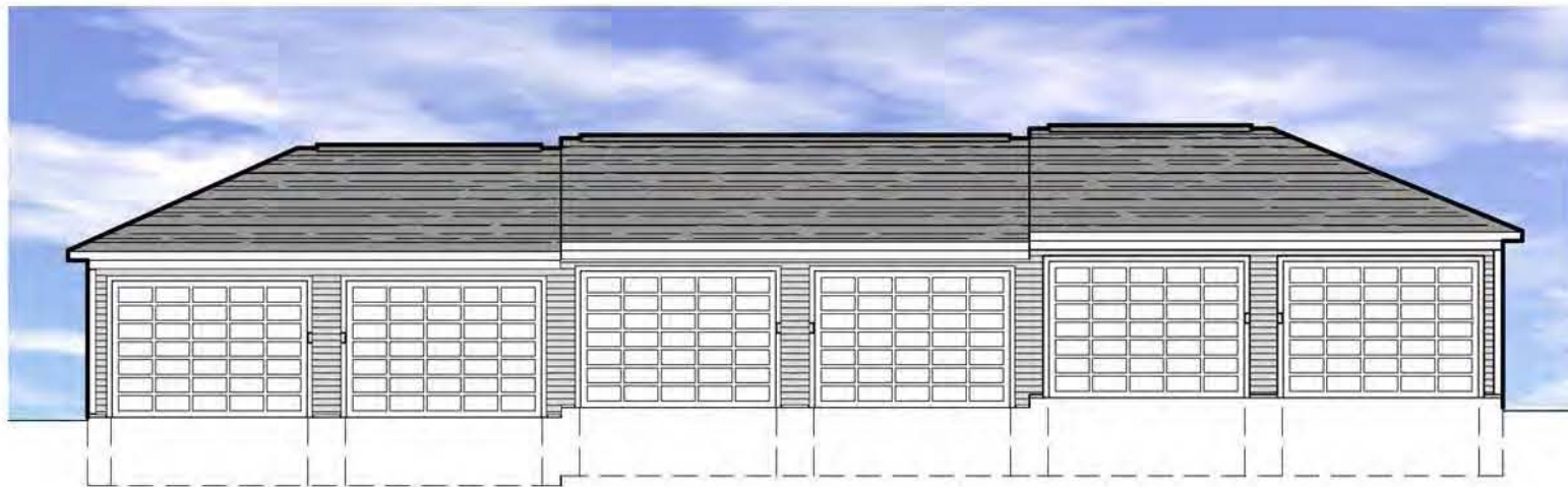
6-Stall Front Elevation w/ 3 Finish Floor Elevations
